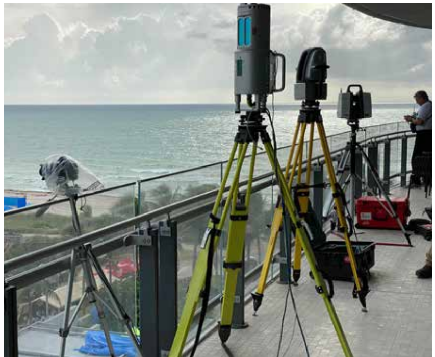
Cameras and lidar equipment are used by NIST, in partnership with USGS and NSF-RAPID researchers, to scan and record conditions at the site of the Champlain Towers South condominium collapse in Surfside, Fla. (Photo courtesy of NIST.)
